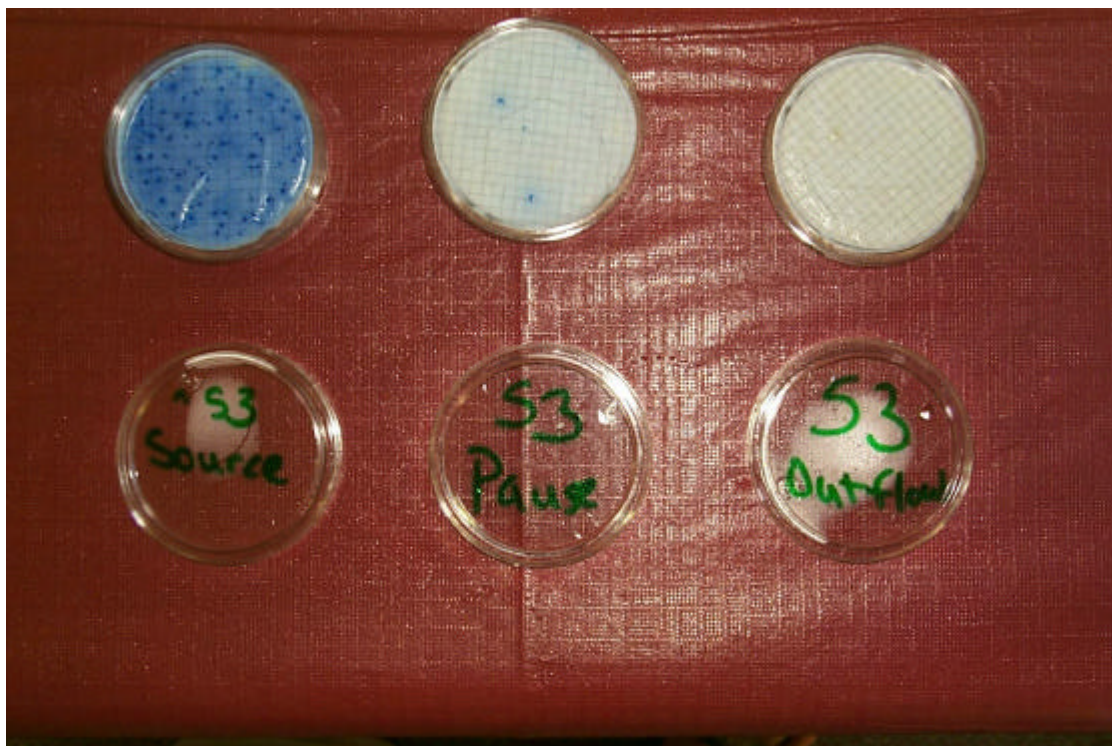
Figure 3: An overhead view of colony forming units in the Source (1450 cfu/100mL), the Pause (30 cfu/100mL) and the Outflow (0 c fu/100mL)
