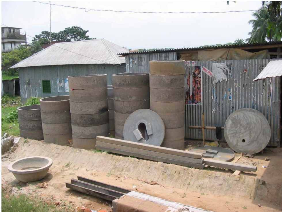
Factory for manufacturing concrete rings and bases for latrines, wells and water storage tanks.
