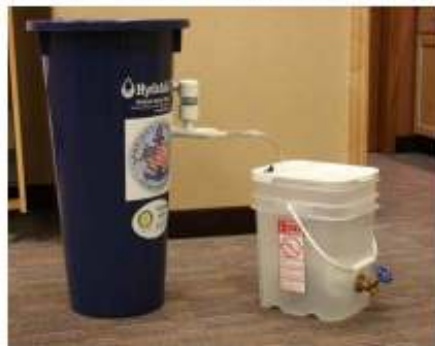
Figure 2 – The HydrAid BSF with chlorinator and safe storage container. This storage container also incorporates a dechlorination device to prevent bad taste and odor.
